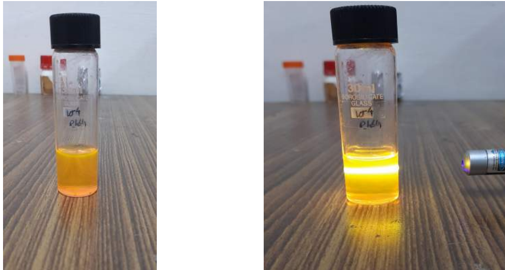
Figure 12: Photographs of carbon quantum dots mixed with red dye solution (a) normal condition and (b) exciting with blue laser.
