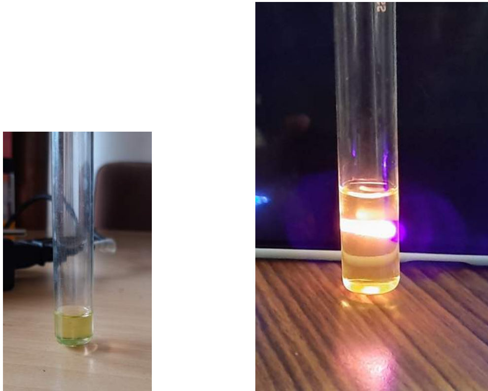
Figure 10: Photographs of carbon quantum dots mixed with the solution of chlorophyll (a) normal condition and (b) exciting with blue laser.
