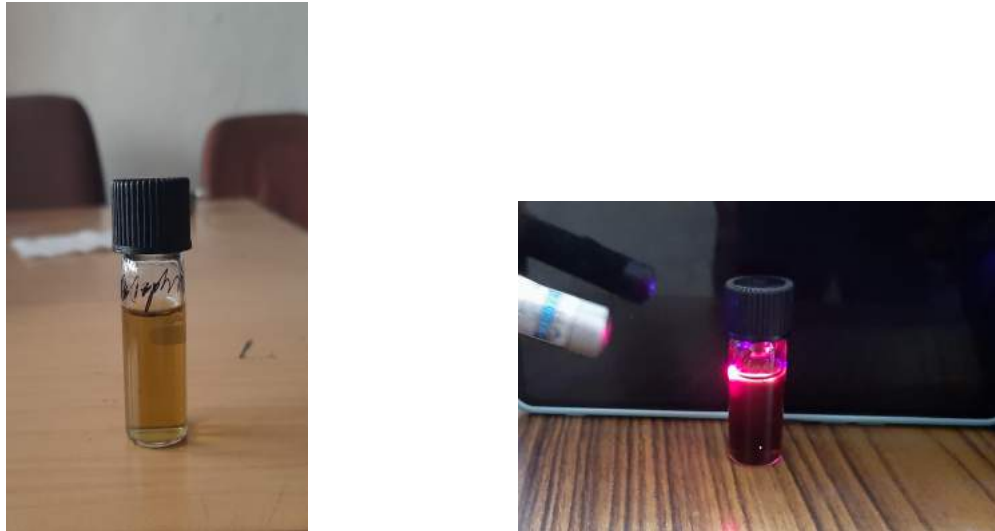
Figure 8: Photographs of mixture of chlorophyll with ethanol in (a) normal condition and (b) exciting with blue laser.
