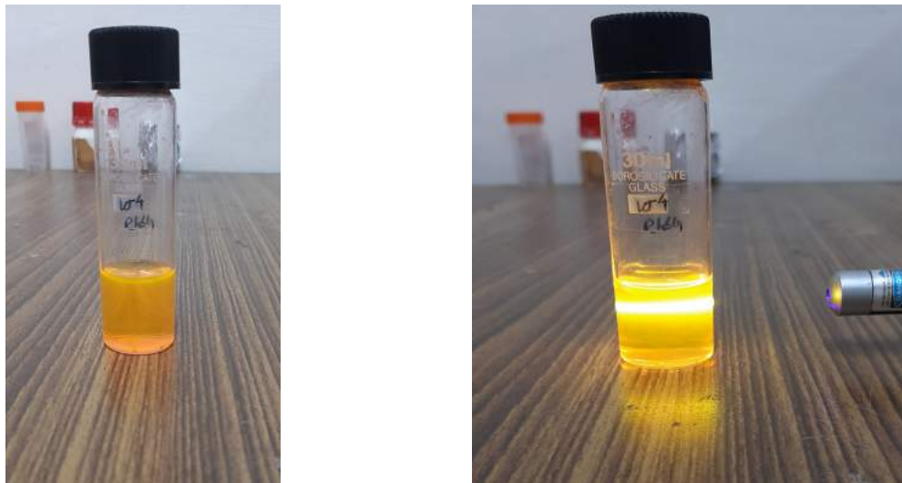
Figure 12: Photographs of carbon quantum dots mixed with red dye solution (a) normal condition and (b) exciting with blue laser.
