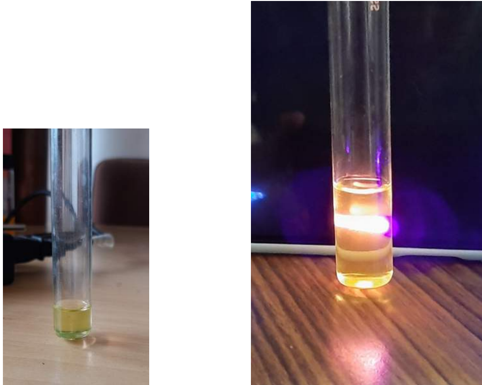
Figure 10: Photographs of carbon quantum dots mixed with the solution of chlorophyll (a) normal condition and (b) exciting with blue laser.
