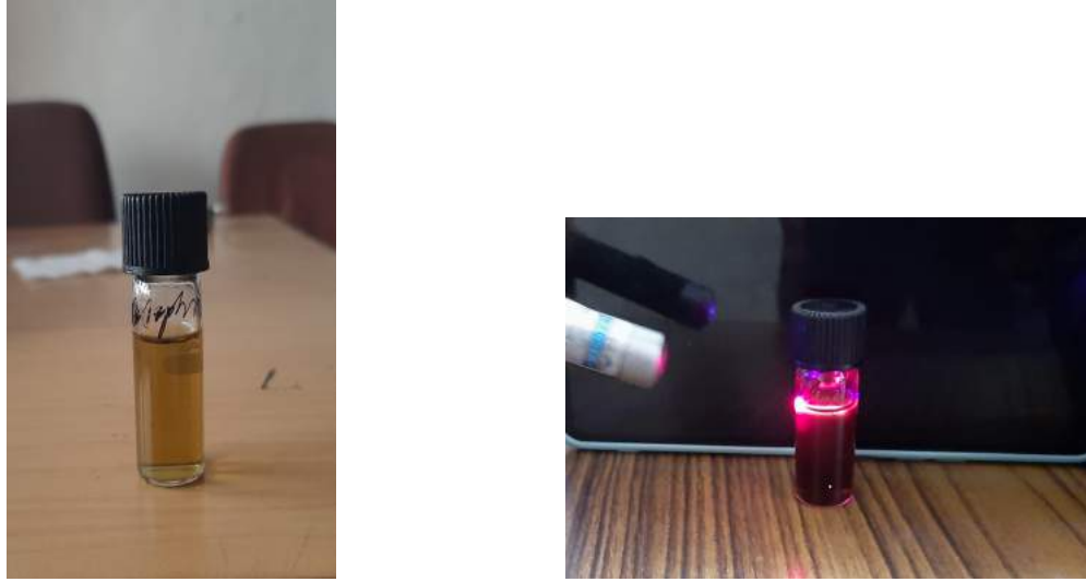
Figure 8: Photographs of mixture of chlorophyll with ethanol in (a) normal condition and (b) exciting with blue laser.
