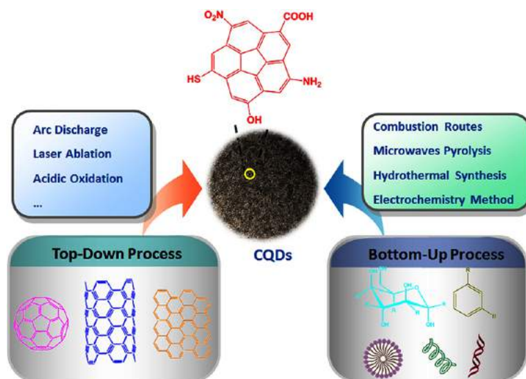
Figure 1: Synthesis Process for Carbon Quantum Dots. [8]
